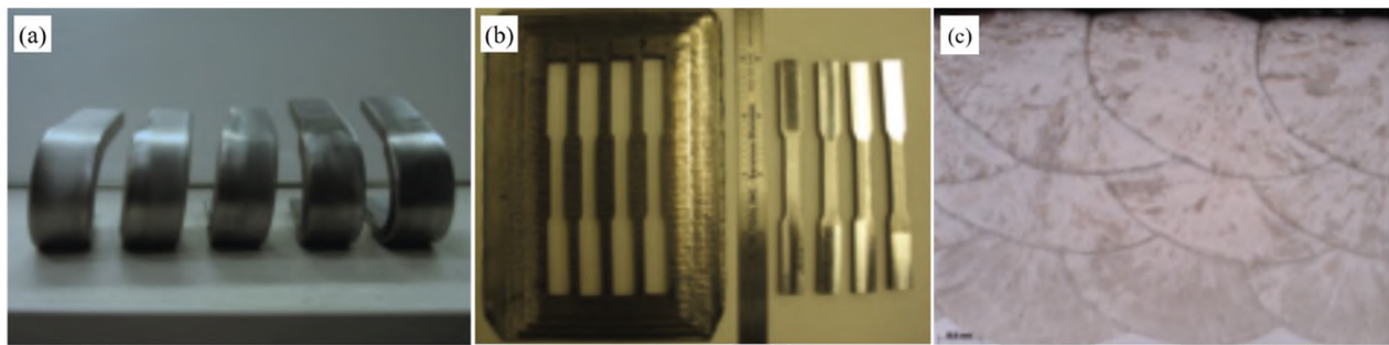
Figure 10 (a) Side-bend test samples, (b) all-weld-metal tensile samples and (c) three-layer ER308L weld on 304L SS plate using the underwater laser beam welding technique [38]
